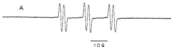
Figure 4. EPR spectrum of product from photolysis of 5, DIPMA, and MNP after HPLC-EPR separation.
